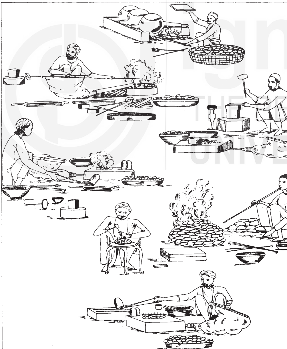
Figure 14.13: Processing of Metal: Smelting; Use of Charcoal; Furnaces; Bellows ( Ain-i Akbari )
