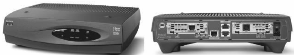
Fig. 2.15: A Common Router with its Front and Back View
